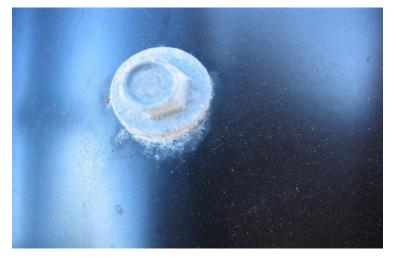
Results of corrosion at Bellambi Point NSW, 10 months exposure
