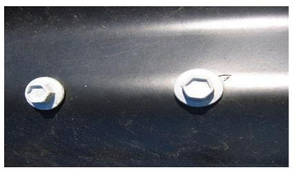
Results of corrosion at Bellambi Point NSW, 10 months exposure
